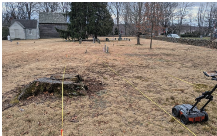
GPR machine and grid lines for the survey conducted by Horsely Archaeological Prospection on January 22, 2020.
