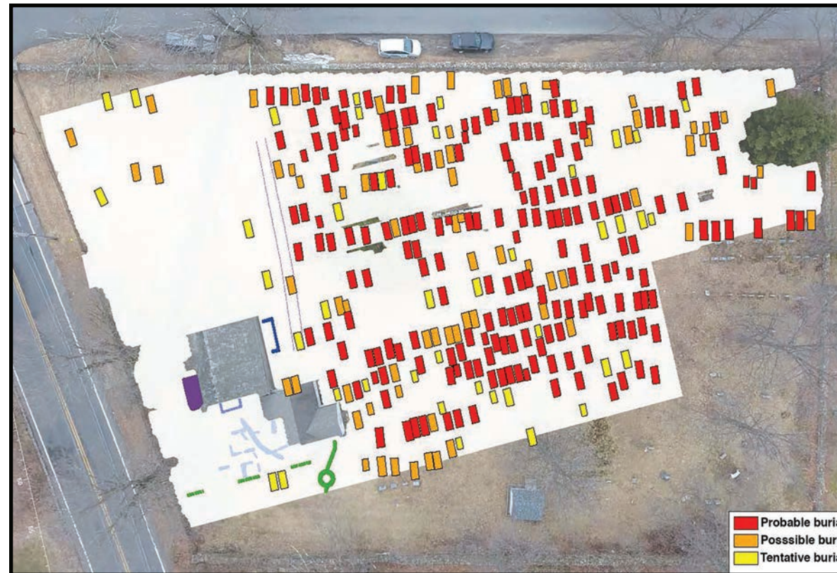
Simplified interpretation of the geophysical anomalies discovered by the January 2020 ground penetrating radar survey, superimposed on a drone photograph of the site taken by Joe Schilip, County College of Morris.
